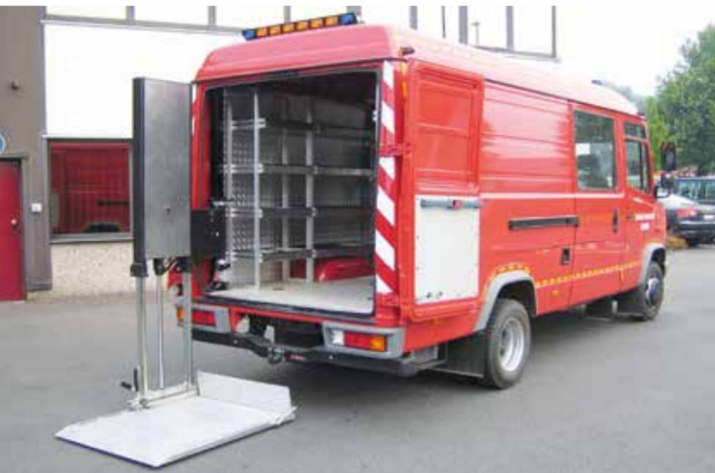
The interior column lift DH-VZ is designed to suit a wide range of Multi Passenger Vehicles, vans, and even larger commercial vehicles.
