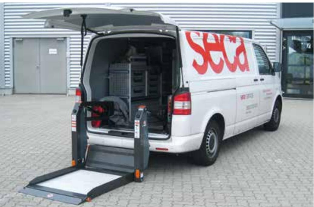
The DH-P2 is a fully automatic linear lift, suitable for mounting **inside the cargo space** of the vehicle. It can be mounted at the rear doors or at the side doors of a wide range of Multi Passenger vehicles and vans.
