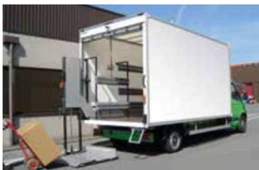
In its travel position, the interior lift **DH-VZS** is stowed against the side of the body and offers the driver **quick and free access** through the vehicle doors. Upon use, the platform is simply pulled out and opened by hand. As the platform slides straight towards the door exit, the floor space beside it can be fully occupied (as opposed to the DH-VZ.03). A wander lead with spiral cable is used to operate the platform up and down.
