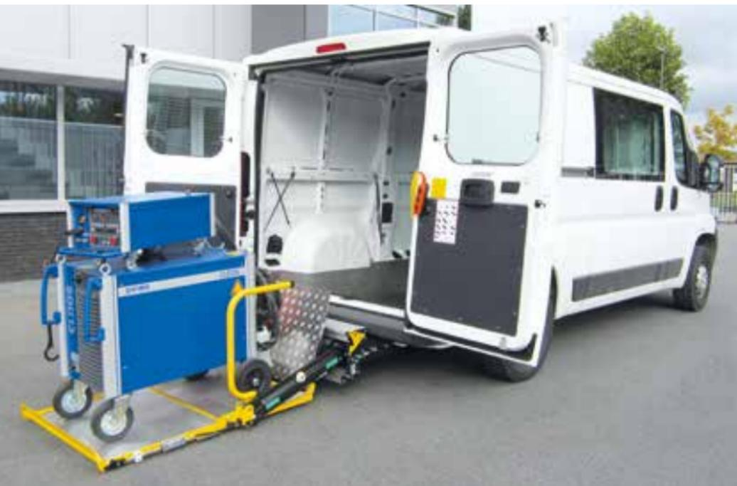
The cassette lift DH-C001 stows neatly in a sealed cassette box under the loading floor of the vehicle. This solution keeps the **access through the rear doors free** and **occupies no space inside the vehicle**.
