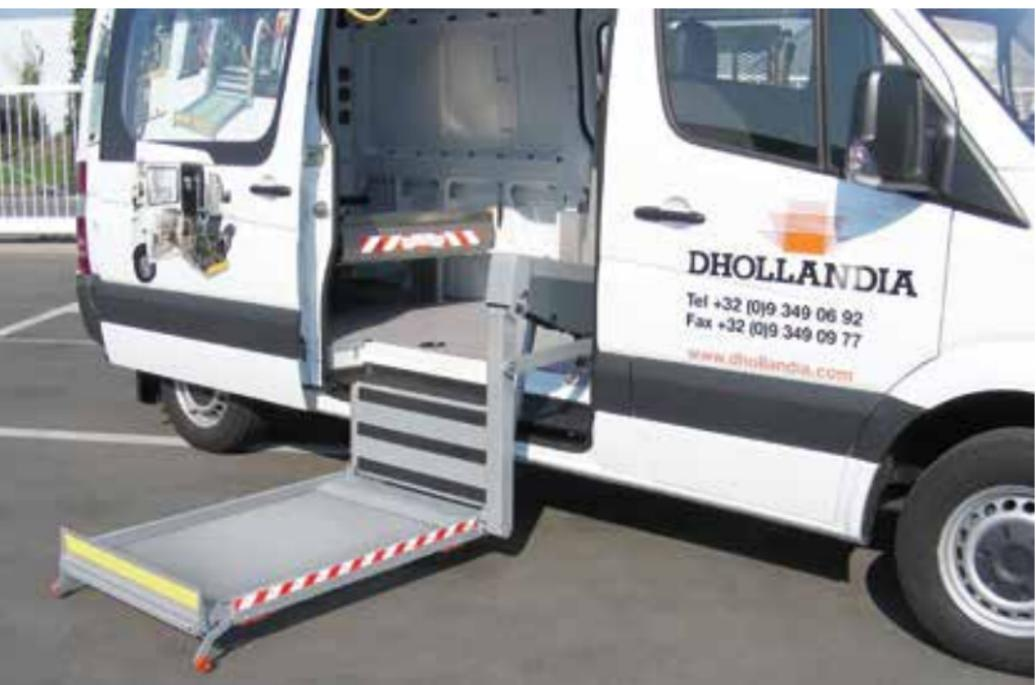
The DH-P1 is a **linear 1-arm lift**, suitable for mounting inside the rear or side doors of a wide range of Multi Passenger Vehicles and vans.
