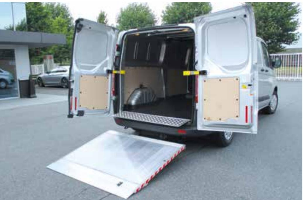
The DH-LSP was the first external lift ever in the tail lift industry, **engineered to suit factory built panel vans**. DHOLLANDIA still continues to lead the innovations in this field today. The intelligent shape of the lift arms **eliminates the need to cut** in the vehicle chassis or rear floor cross member, and **maximises the ground clearance** under the lift.
