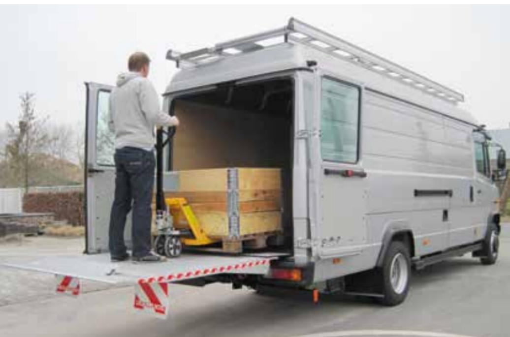
The DH-LC.15 offers 1500 kg lift capacity for the **higher capacity factory built panel vans** from 4.5 up to 7.5T GVW (e.g. Mercedes Vario, Iveco Daily,...).
