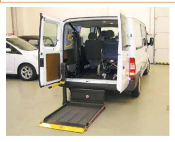
The DH-PH1 is a **linear 1-arm lift**, suitable for mounting inside the rear or side doors of a wide range of Multi Passenger Vehicles, minibuses and ambulance vehicles.
