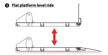
The platform remains level during the full lifting / lowering cycles. The rear end of the platform can be a fixed leading edge, or hinged ramps which adjust more easily to uneven surfaces.
