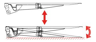
When lowering, the platform remains level from the vehicle floor down until the platform rollers touch the ground. Next, the platform tilts down to an inclined position that allows loading and unloading.
