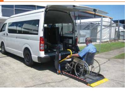
The DH-PH2 belongs to a new generation (2010-...) of **fully automatic linear passenger lifts**. It is suitable for mounting inside the rear doors of a wide range of Multi Passenger Vehicles, minibuses and ambulance vehicles.
