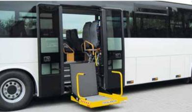
The DH-CH100...103 are **heavy duty cassette lifts**, to assist wheelchair passengers to embark or disembark the midibus or coach in optimum safety.
