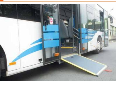
The access ramps DH-BRM... are designed to assist wheelchair passengers, parents with a baby buggy, or passengers with an otherwise impaired mobility to enter or exit the bus safely and comfortably.
