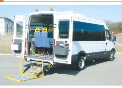
The passenger lift DH-CH001 stows neatly in a sealed cassette box under the loading floor of the vehicle. This solution keeps the access through the rear doors free and occupies no space inside the vehicle.
