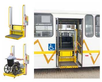
The **DH-TV 300 kg** is specially designed for **urban buses**, to assist wheelchair passengers to embark and disembark the vehicle in a comfortable and safe manner.
