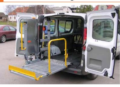
The interior column lift DH-VZH is designed to suit a wide range of Multi Passenger Vehicles, minibuses, coaches, trains, ...
