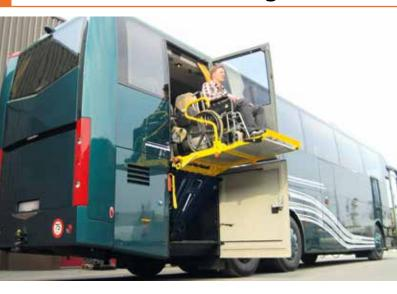
The **fold-away** lift DH-RB is specially designed for coaches, to help wheelchair passengers to embark and disembark the vehicle in a comfortable and safe manner.
