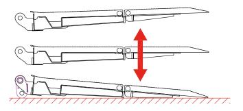
When lowering, the platform progressively tilts down from a level position at the vehicle floor to an inclined position at the ground. (And vice versa when lifting).
