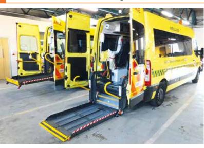
The reinforced linear 2-arm lift offers 500 kg lift capacity and fulfills the most demanding requirements of the passenger transport sector. The platform depth can be extended to 1600 mm to load and unload hospital stretchers. The platform width can be increased to 920 mm to suit bariatric applications, both wheelchairs and stretchers.
