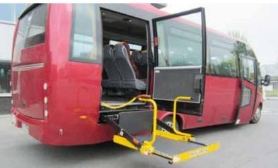
In comparison to the DH-CH100...103, the DH-CH002 and -CH003 are equipped with **extensible platforms**, significantly **reducing the required fitting space** under or inside the vehicle.
